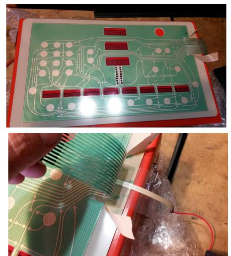
7. Begin placing the membrane on the console by carefully inserting the shield wire and ribbon into the slot in the setworks console.
