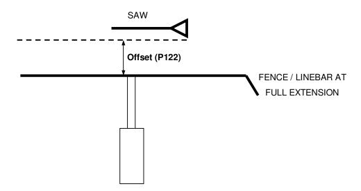
Figure 5.1: Bird's eye view of the breast-bench / resaw ram
