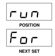
After the "C" function has been selected, the displays in the centre of the console will appear as shown above. The operator will then press Enter to initiate the function. The drive signal will then be applied to the forward valve until the Clear button is pressed.
