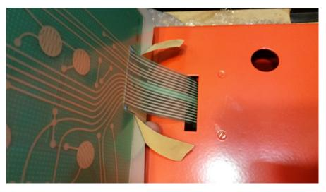
8. Once the ribbon and shield wire are through the slot position the membrane over the console aligned with the outside marking made previously. Attempt to lay the membrane on the console from the opposite side of the ribbon first, then before the ribbon side is laid on the console, remove the last piece of the protective backing from under the ribbon.
